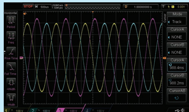
Three Phase Unbalance Voltage Test Captured
